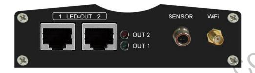
[1 LED-OUT 2] Connect to the receiving card's Gigabit Ethernet port;
